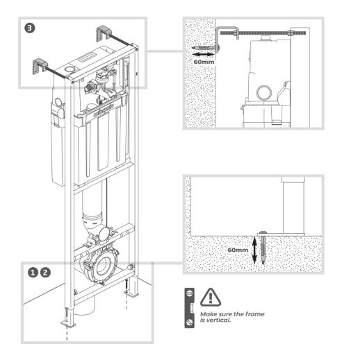
**EN 3** Mark and drill the hole for the feet mountings. **2** Secure using screw (v) and plug (w). **3** Position the wall brackets (w), and threaded rods (w) and fix them to the wall with (w), (v) and (w). Cut the rod if required. **3** Make sure the frame is vertical by tightening or loosening the nuts (w).
