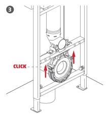
exi ① Position the frame and WC pan connector (h) and mark the cutout if necessary. If required, measure, cut and deburr the WC pan connector. Make sure to remove the seal and carefully reposition it after cutting. ② Push fit the WC pan connector in place. ③ Secure the WC pan connector into the bracket.
