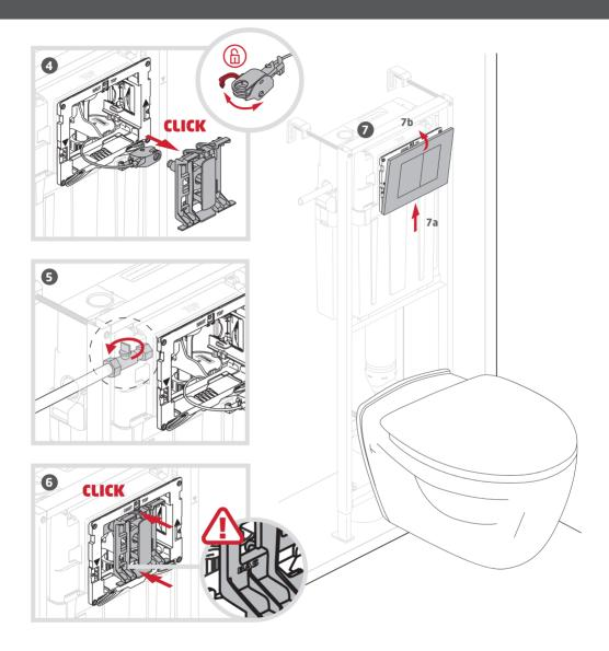
EN ① Remove the cardboard protection and cut the access channel flush against the wall. ② Insert the push plate bracket ② in the access channel, paying attention to the installation direction. ③ Secure with clips ③. ③ Clip the flush valve cable to the push plate connector ⑥. ⑤ Open the isolation valve.
