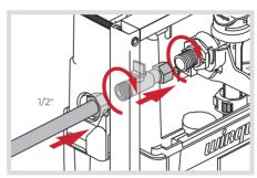
IN Uncap the opening on the left of the frame. (Top and rear feed possible, taking care not to interfere with the cable control). Attach the shut-off valve (v) to the inlet valve installed in the cistern. Connect to the external water supply.
