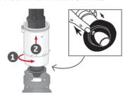
We recommend that you service your flush valve sealing washer every 5 years. Remove the flush valve by turning 1/4 turn, remove the sealing washer as shown and clean with soapy water before repositioning. Insert the flush valve into the base and secure it with a quarter-turn clockwise.
