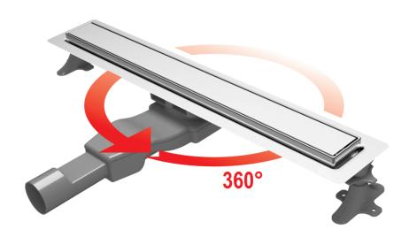
Flat stainless steel shower channel with 360° rotative PP drain. It is compatible with tiles from 13 to 23 mm and its feet are adjustable from 62 to 85 mm. Waterproofing fleece is included and perfectly adjustable on the stainless steel flange!
