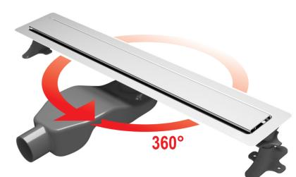
Stainless steel shower channel with 360° rotative PP drain. It is compatible with tiles from 9 to 19 mm and its feet are adjustable from 75 to 85 mm. Waterproofing fleece is included and perfectly adjustable on the stainless steel flange !
